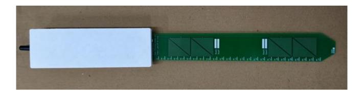
**IOT Enabled Soil Moisture probe:** We have developed soil moisture sensor based on fringing electric field (FEF) technology to measure the soil moisture in the crop field and optimize the irrigation process. This technology provides good accuracy at required measurement range of soil moisture content and is also cost effective. The probe can measure soil moisture at multiple depths.
